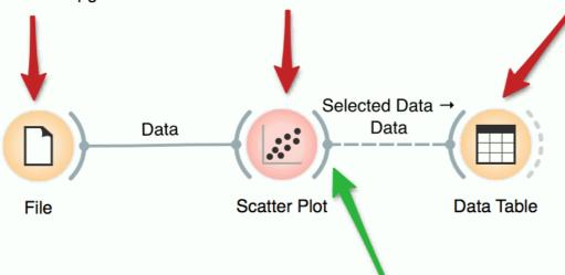
Try to connect some other widget to the output of the Scatter Plot. Say, a Box Plot widget (toolbox, Visualize pane). Box Plot will display distributions of the data subset selected in the Scatter Plot.
